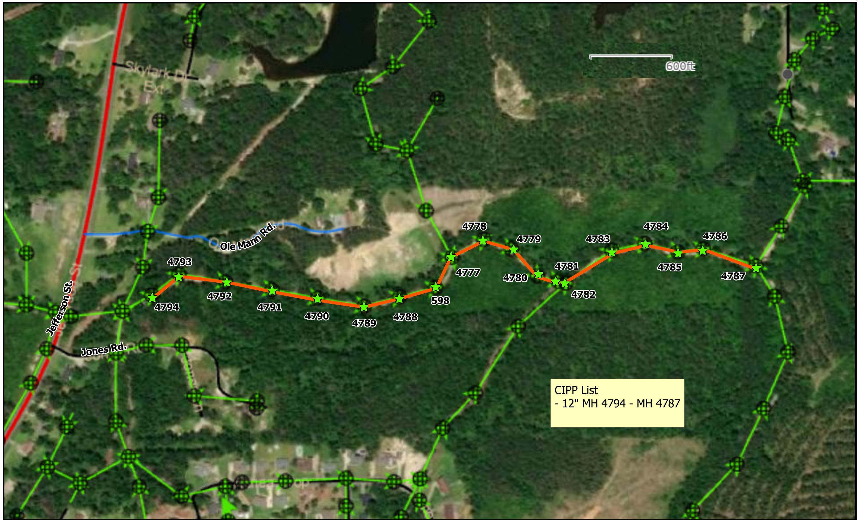
Figure 3 2022 Annual Sewer Maintenance and Rehabilitation Project Jones Village to Voss Rd. Line City of Alexander City, AL
